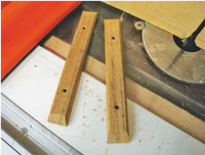
▲ Pic.11 He rounded over the edges of the two sides of the handle on a router table
